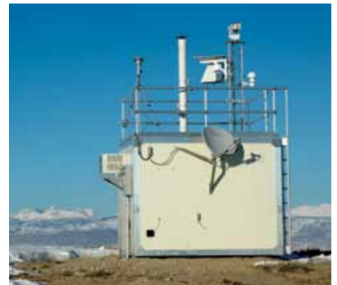
The Boulder air monitoring station in Sublette County, funded jointly by the operators and the Wyoming Department of Environmental Quality (WDEQ), monitors ambient air quality downwind from the field.
