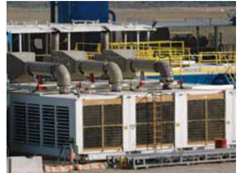
We're using Selective Catalyst Reduction (SCR) technology on many of the field's drilling rigs.
